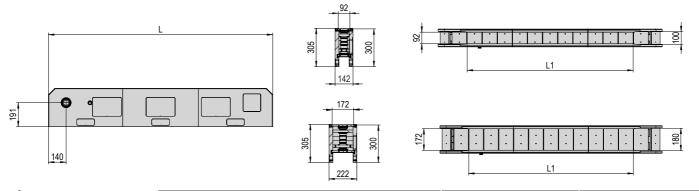
**The LTM** consists of a drive module, deflection module and 0 to 5 middle modules.
